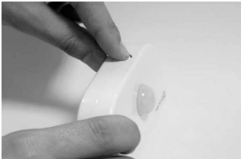
In order to mount the detector in a corner, place the corner mounting bracket provided with the equipment in the desired location. Use a pencil to mark the location of the fixing screw holes.
